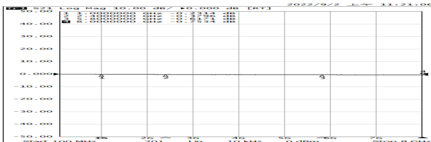
Channel 1 - Insertion Loss
